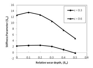
${\bf Figure \ 9} \ {\rm Direct \ fluid-film \ stiffness \ coefficient \ versus \ relative \ wear \ depth}$
