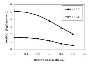
Figure 5 Load carrying capacity versus relative wear depth
