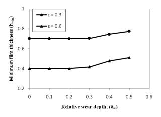
Figure 4 Minimum fluid-film thickness versus relative wear depth
