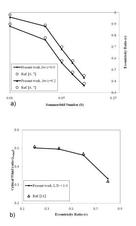
Figure 3 a) Eccentricity ratio versus Sommerfeld number, b) Critical Whirl ratio versus Eccentricity ratio
