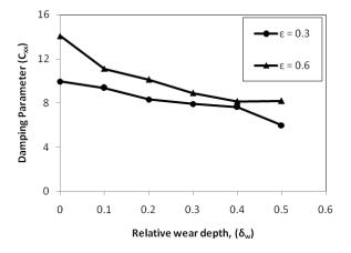
Figure 10 Direct fluid-film damping coefficient versus relative wear depth
