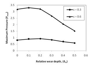
Figure 6 Maximum pressure versus relative wear depth
