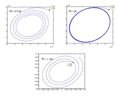
Figure 12 Non linear trajectories for hydrodynamic journal bearings at eccentricity ratio of 0.3 and  $\bar{\delta}_w = 0.0$
