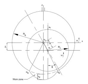
Figure 1 Worn bearing geometry
