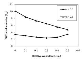
Figure 8 Direct fluid-film stiffness coefficient versus relative wear depth
