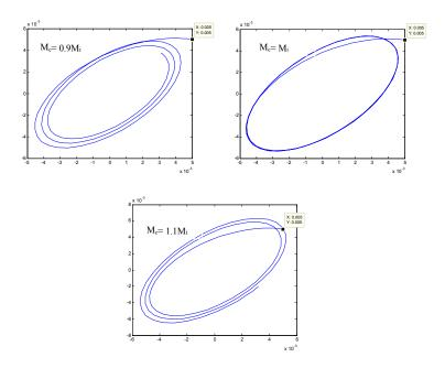
Figure 15 Nonlinear trajectories for hydrodynamic journal bearings at eccentricity ratio of 0.6 and  $\bar{\delta}_w = 0.0$
