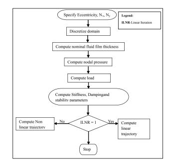
Figure 2 Overall solution process scheme
