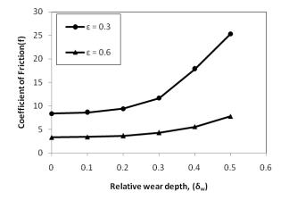
Figure 7 Coefficient of friction versus relative wear depth
