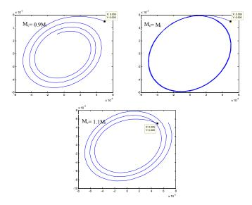
Figure 13 Non linear trajectories for hydrodynamic journal bearings at eccentricity ratio of 0.3 and  $\bar{\delta}_w = 0.2$
