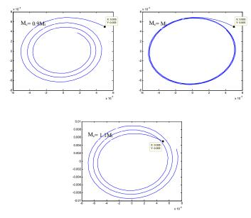
Figure 14 Nonlinear trajectories for hydrodynamic journal bearings at eccentricity ratio of 0.3 and  $\bar{\delta}_w=0.4$
