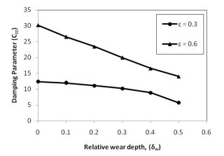
${\bf Figure \ 11} \ {\rm Direct \ fluid-film \ damping \ coefficient \ versus \ relative \ wear \ depth}$
