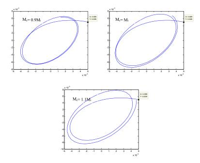
Figure 17 Nonlinear trajectories for hydrodynamic journal bearings at eccentricity ratio of 0.6 and  $\bar{\delta}_w=0.4$
